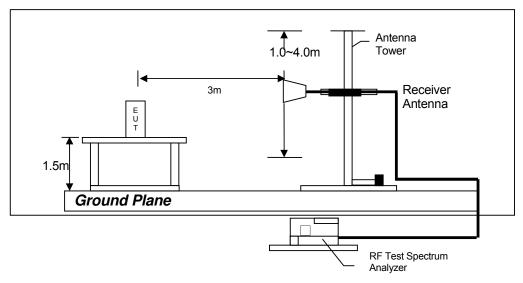
Test setup of radiated emissions above 1GHz
