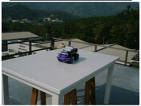
MEASUREMENT OF RADIATED EMISSION TEST SET UP
