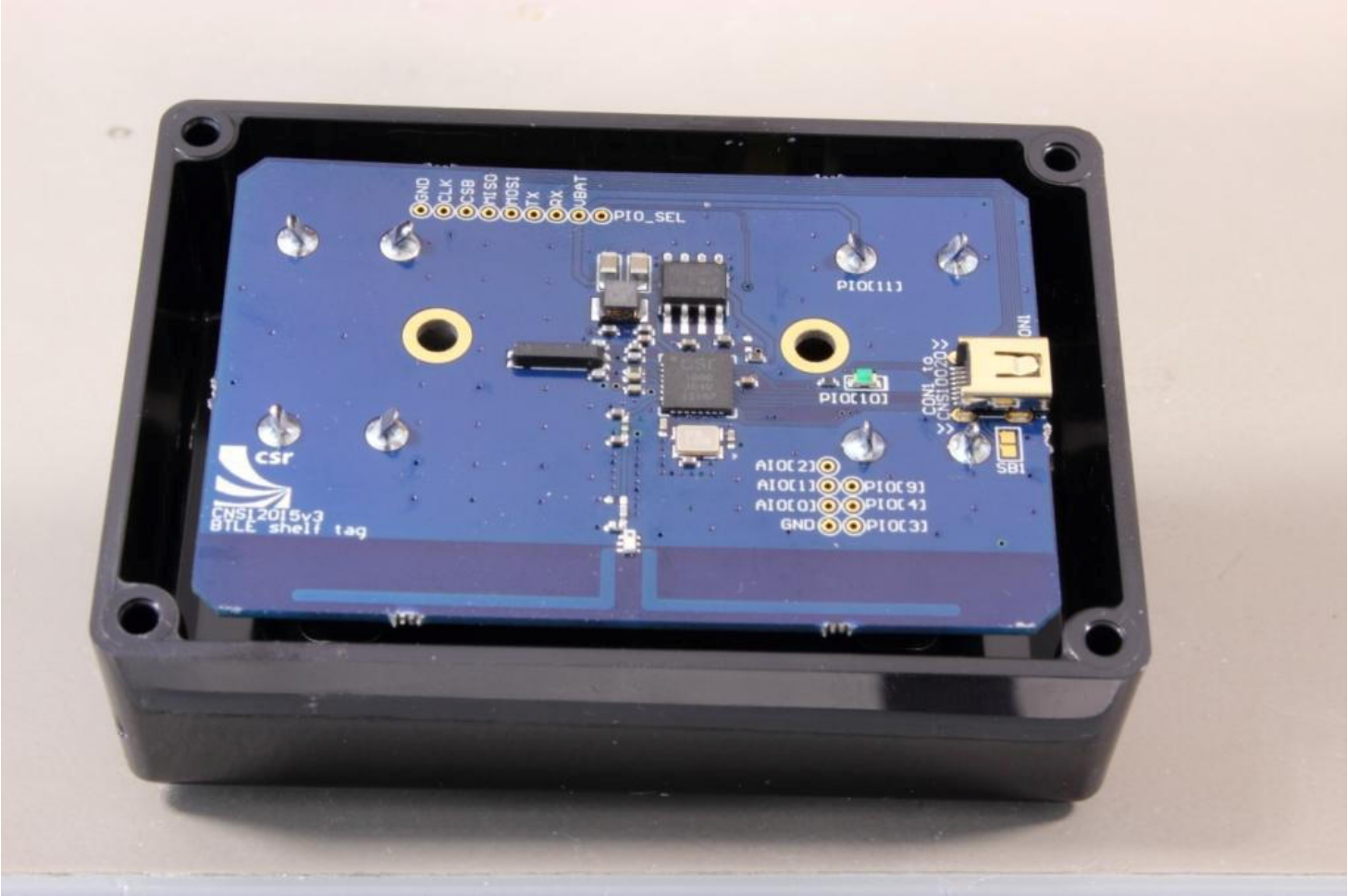
PCB mounted in box, no lid.
