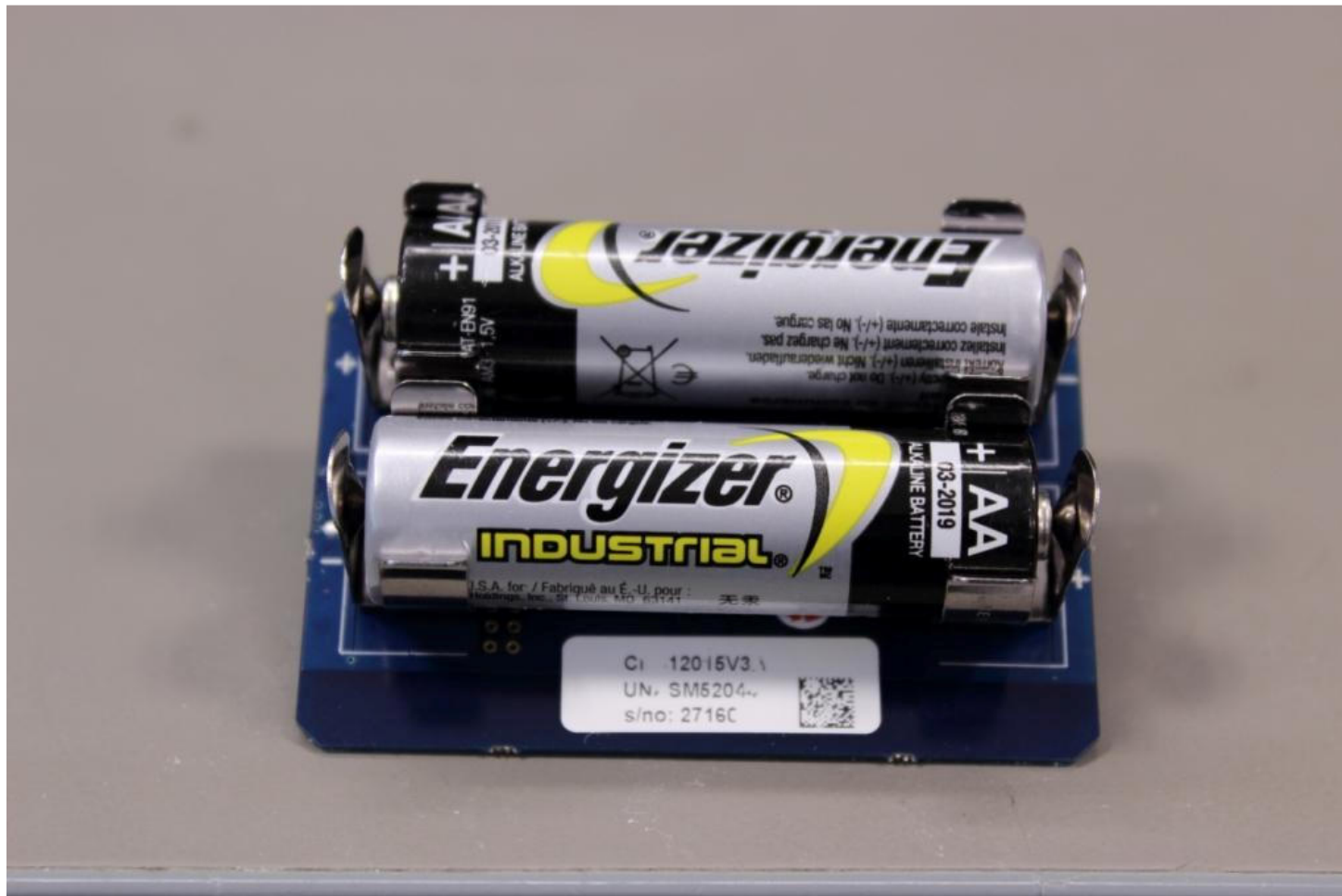
PCB Rear - Batteries mounted
