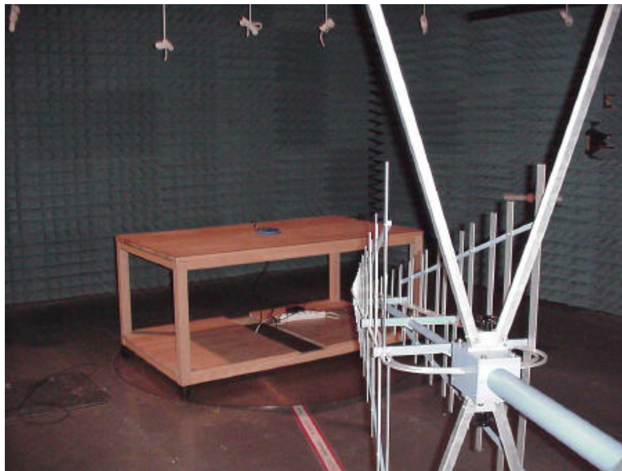
Picture 1 : Setup for radiated emission test, front view
