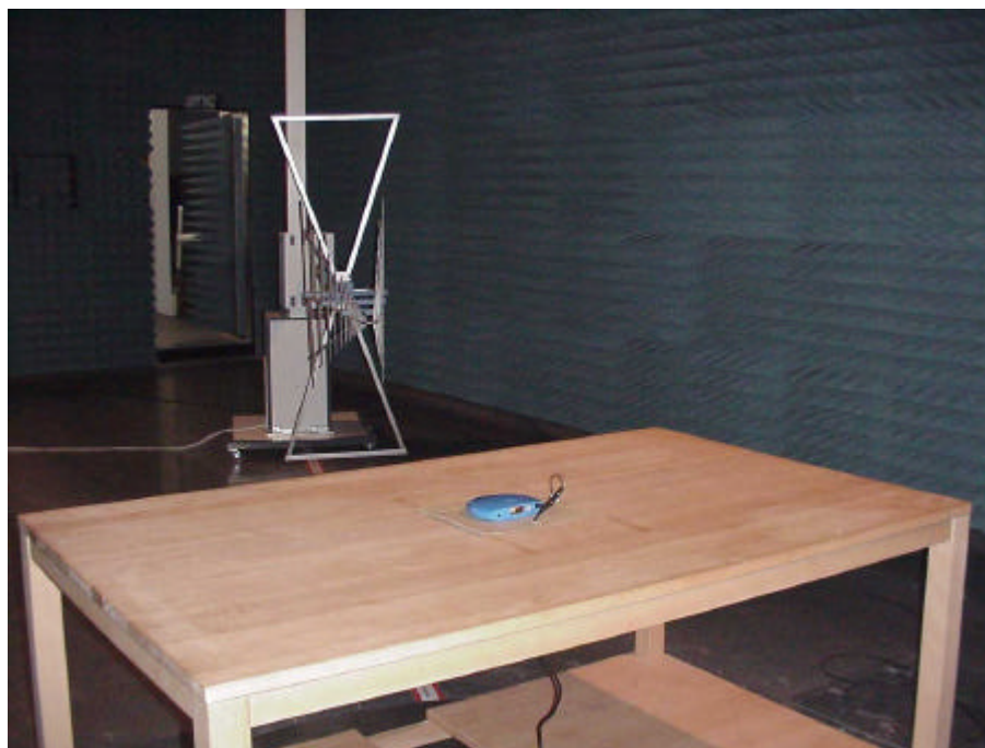
Picture 2 : Setup for radiated emission test, rear view
