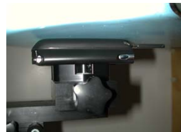
Figure 19. Hand SAR Test Setup
