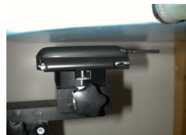
Figure 17. Body SAR Test Setup
