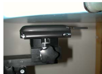
Figure 16. Body SAR Test Setup
