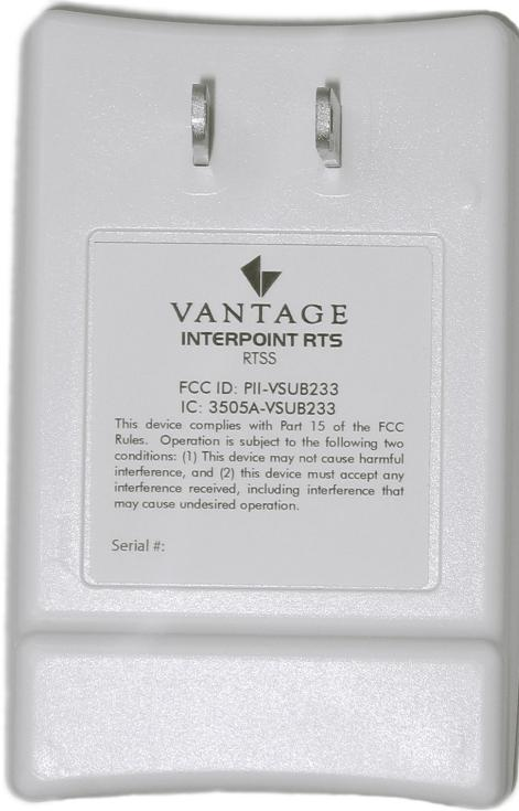
The label is placed on the back of the case. All InterPoint RTS units will be labeled with a label containing the following wording:
