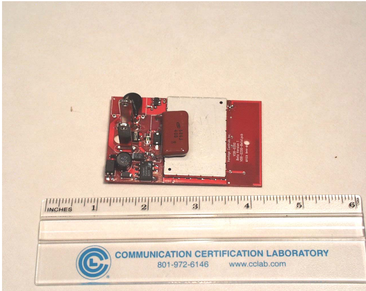
Photograph 7 - Component Side of the PCB with Shield in Place
