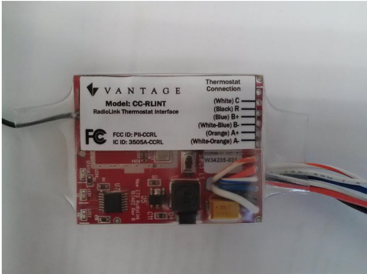
Front View of the EUT with heatshrink in place
