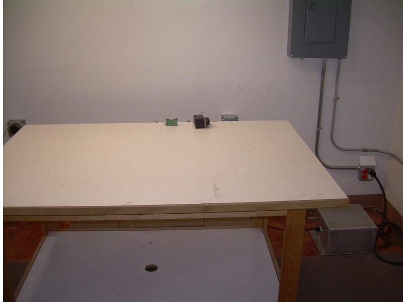
Photograph 11 – Front View Conducted Emissions Worst-Case Configuration
