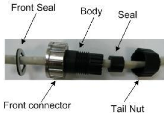
Figure 27 – Ethernet connector cable termination
