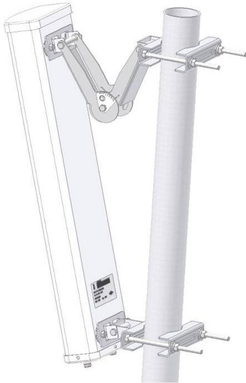
Figure 17 - uMAXe Antenna Dual Slant Mast Mount Configuration
