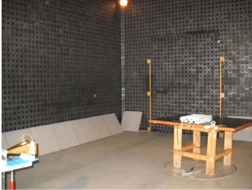
Photograph No.7 Radiated emissions measurement setup in the anechoic chamber in 18 –40 GHz range
