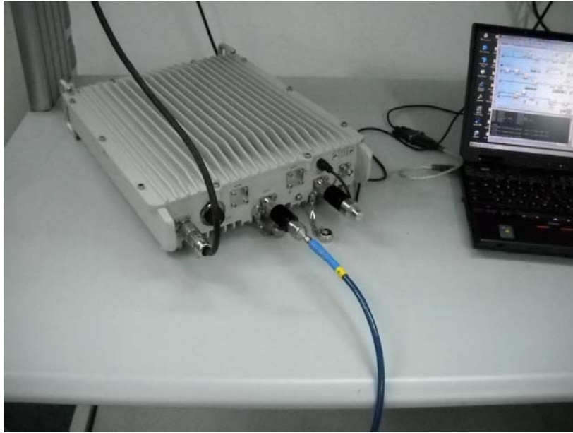
Photograph No.3 Conducted spurious emissions measurement setup
