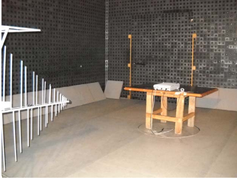
Photograph No.5 Spurious emissions measurement setup in the anechoic chamber in 30 -1000 MHz
