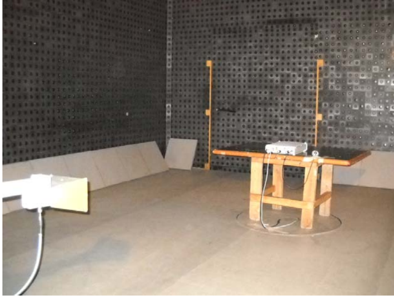
Photograph No.6 Radiated emissions measurement setup in the anechoic chamber in 1-18 GHz range
