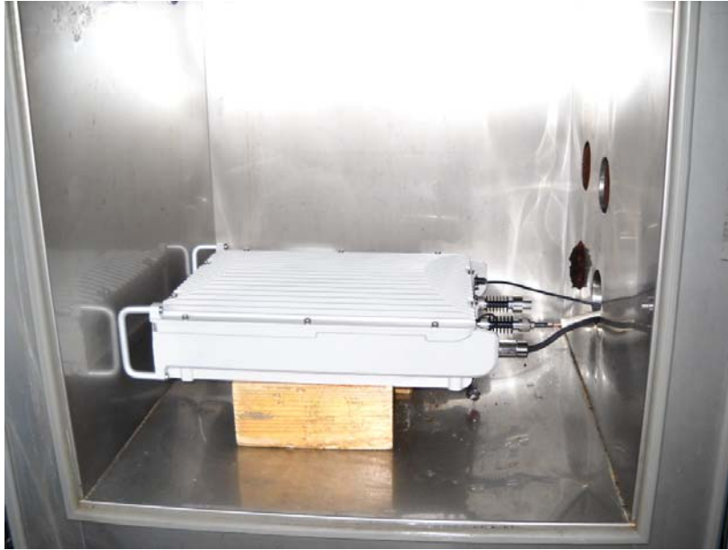
Photograph No.8 Frequency stability measurement setup
