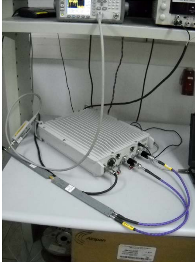
Photograph No.2 Spectral power density, occupied bandwidth, emission mask measurement setup
