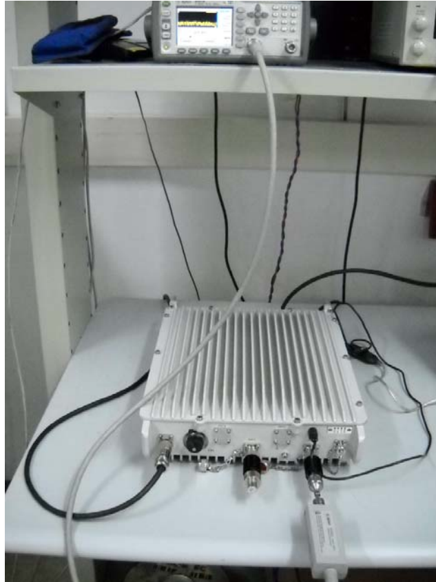
Photograph No.1 Peak output power setup
