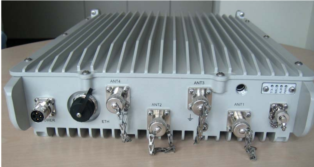
Photograph No.1 “uMAXe/AirGrid 3.65 GHz” base station front view
