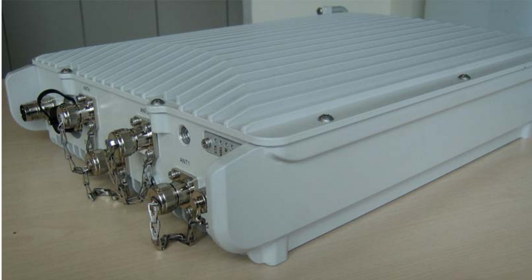
Photograph No.4 “uMAXe/AirGrid 3.65 GHz” base station side panel view
