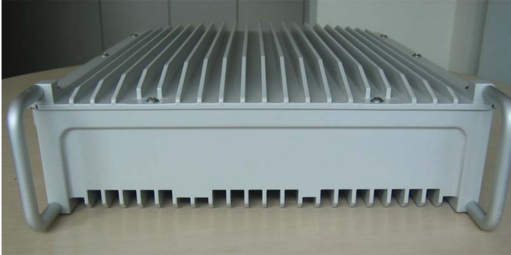
Photograph No.2 “uMAXe/AirGrid 3.65 GHz” base station rear panel view
