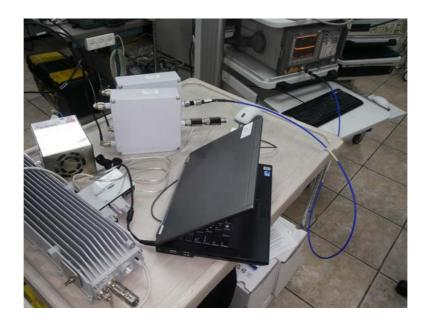
Photograph No.6 Conducted spurious emissions measurement setup
