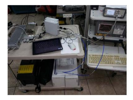
Photograph No.5 Band edge emissions measurement setup
