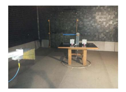
Photograph No.9 Spurious emissions measurement setup in the anechoic chamber above 1 GHz
