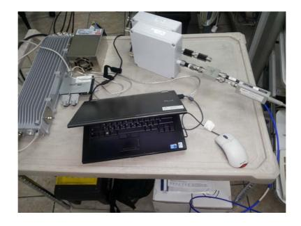
Photograph No.2 Peak output power measurement setup
