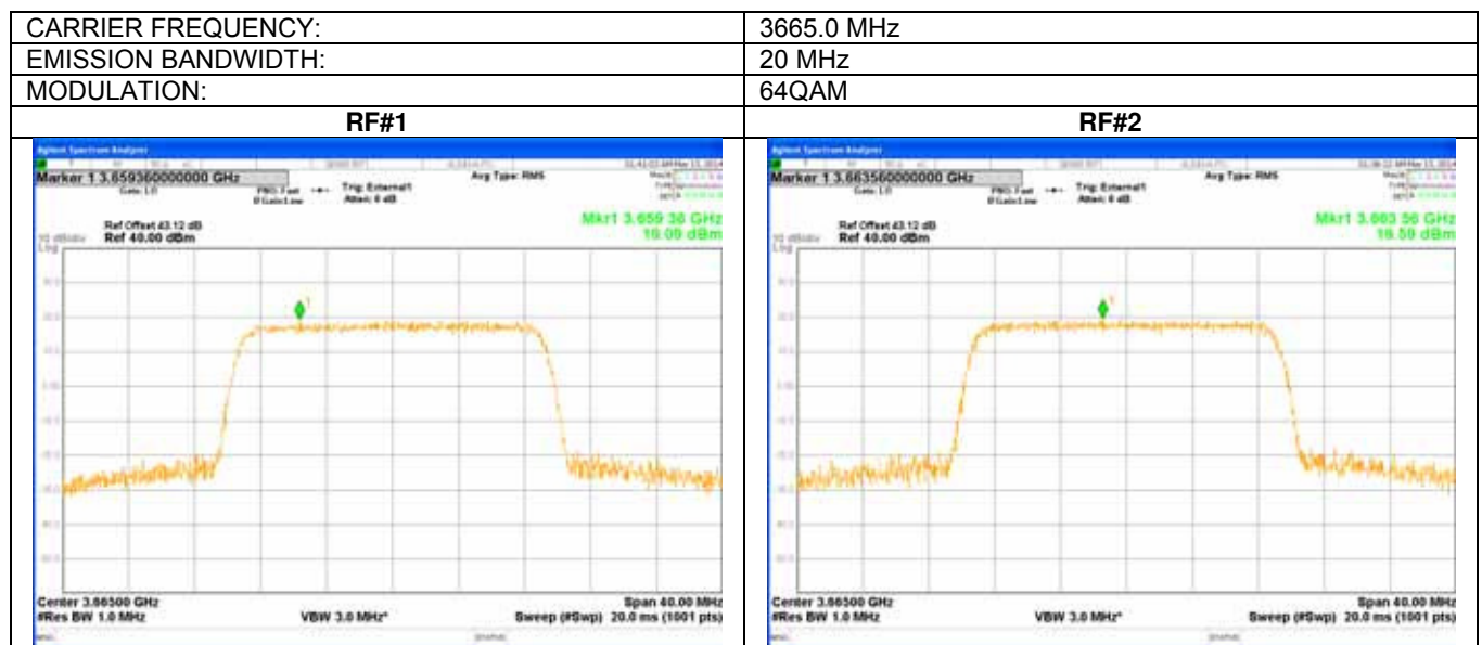
Plot 7.1.12 Peak output power test results at high frequency
