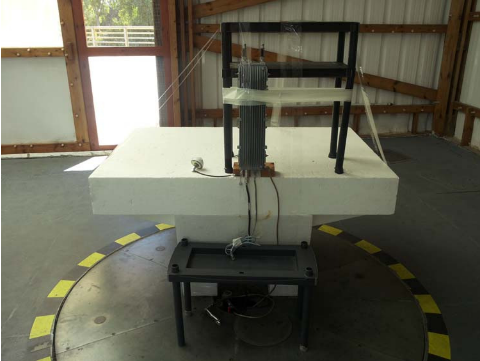
Photograph No.11 Spurious emissions measurement setup at the OATS, EUT close view
