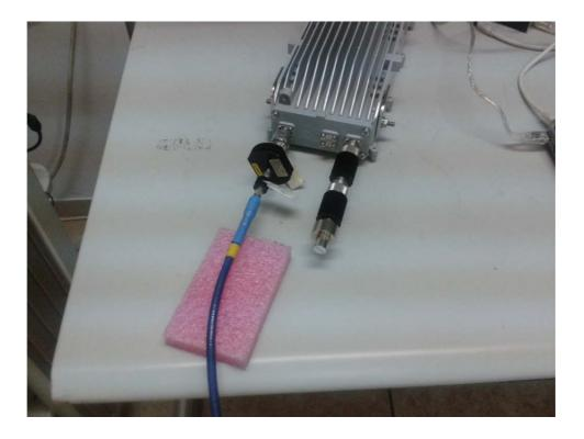
Photograph No.2 Conducted spurious emissions measurement setup
