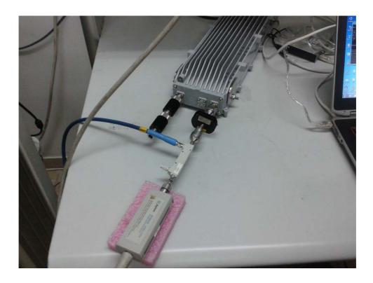
Photograph No.1 Peak output power, OBW, band edge emissions measurement setup
