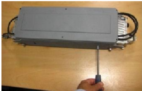
Figure 18 – Attaching front mount antenna assembly to AirSynergy
