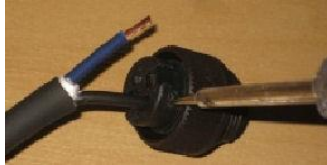
Figure 38 - secure cable to connector
