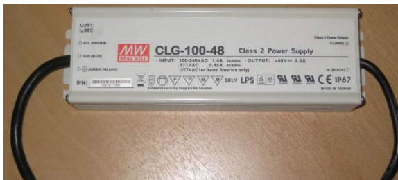
Figure 47 - Standard power (150W) PSU – used for standard AirSynergy installation
