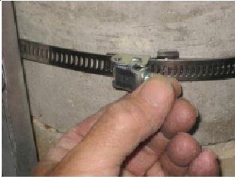
Figure 12 – press down locking mechanism
