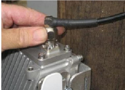
Figure 27 - Connecting RF cable
