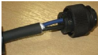
Figure 39 – power cable wires assembled
