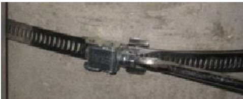
Figure 13 – tighten clamp bands
