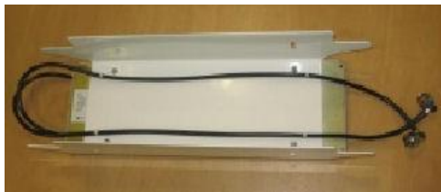
Figure 17 - attaching front mounted antenna to mounting plate
