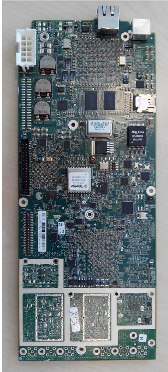
Photograph No.4 SDR-Qc, Digital and RF card front view
