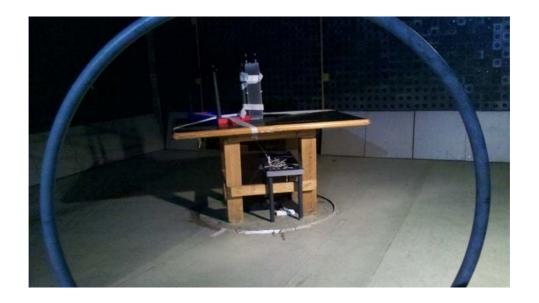
Photograph No.4 Spurious emissions measurement setup in the anechoic chamber in 30 -1000 MHz
