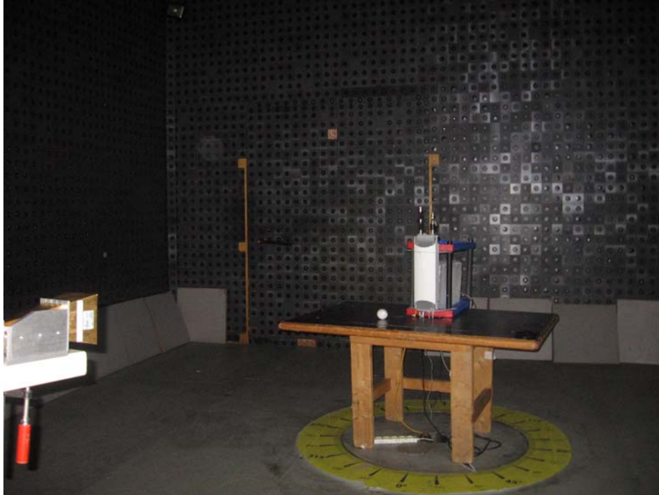
Photograph No.7 Spurious emissions measurement setup in the anechoic chamber in 18-20 GHz
