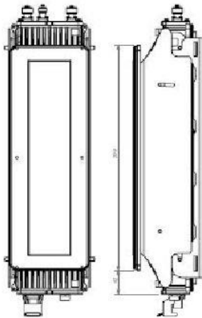
Figure 2 - AirSynergy with front sector antenna
