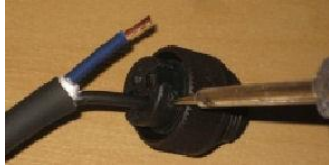
Figure 40 - secure cable to connector
