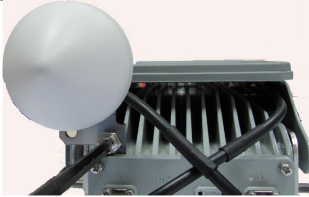
Figure 20 - Attaching the GPS antenna assembly to AirSynergy
