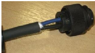
Figure 41 – power cable wires assembled
