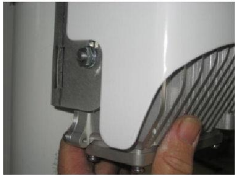
Figure 24 - AirSynergy unit engaged into the bottom slots
