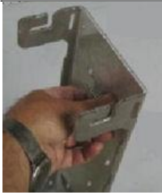
Figure 15 - positioning wall mounting plate
