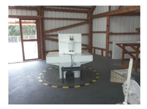
Photograph No.8 Spurious emissions measurement setup at the OATS in 18-20 GHz
