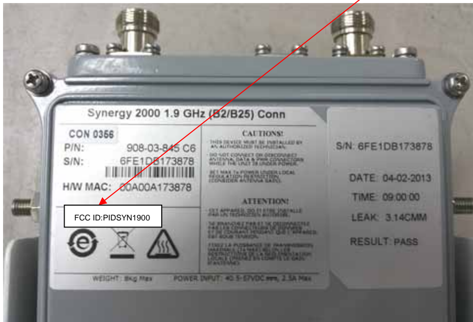
“Synergy 2000, 1.9 GHz” bottom panel, label with FCC ID:PIDSYN1900 location
