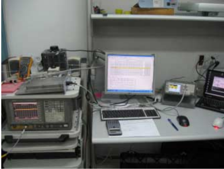
Photograph No.1 Peak output power, occupied bandwidth, emission mask and conducted spurious emissions measurement setup
