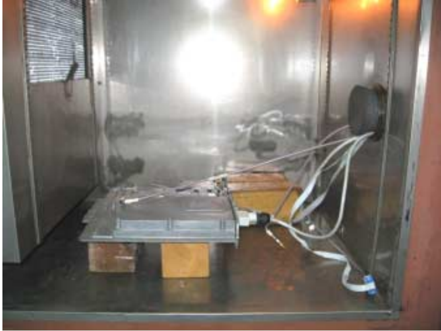
Photograph No.9 Frequency stability measurement setup
