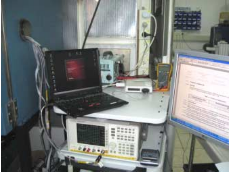
Photograph No.8 Frequency stability measurement setup
