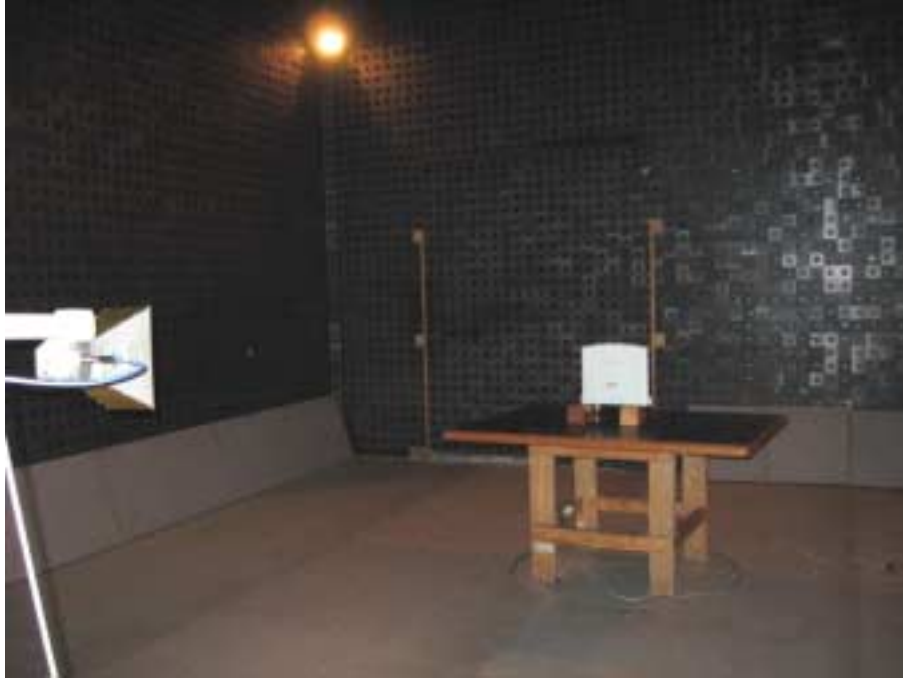
Photograph No.5 Radiated emissions measurement setup in the anechoic chamber above 1000 MHz
