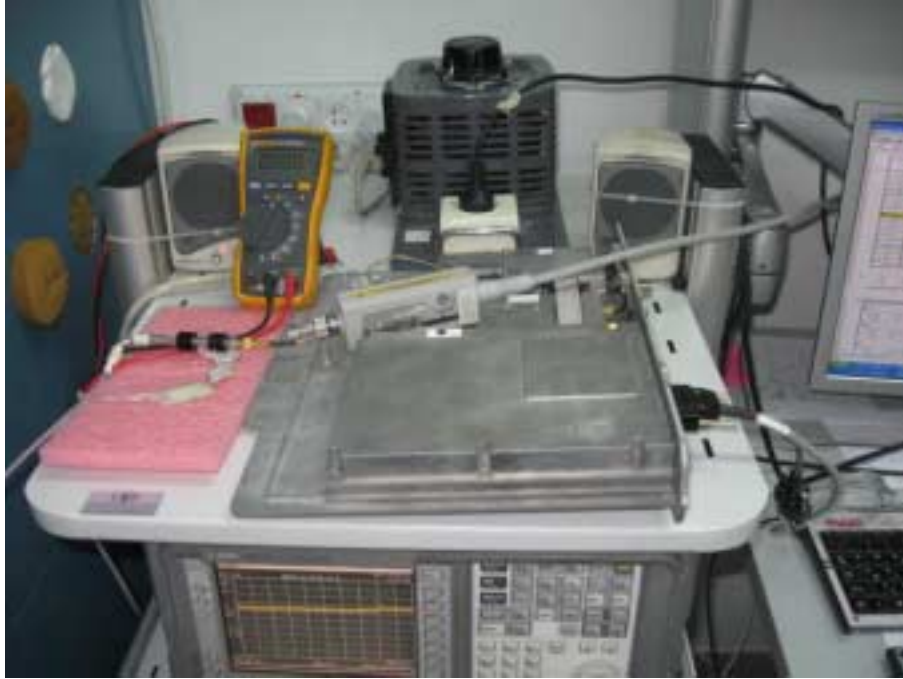
Photograph No.2 Peak output power, occupied bandwidth, emission mask and conducted spurious emissions measurement setup
