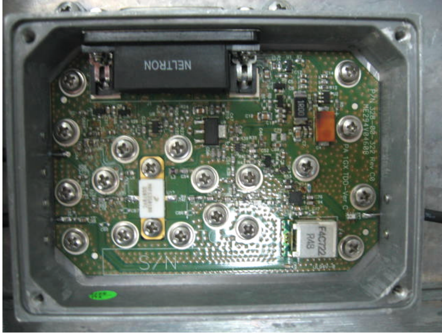
Photograph No.12 Power amplifier (PA) internal view
