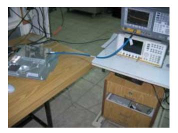
Photograph No.2 Spurious emissions measurement setup in the anechoic chamber above 2900 MHz
