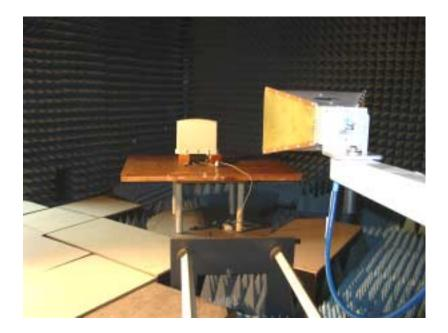
Photograph No.5 Spurious emissions measurement setup an the OATS above 2900 MHz
