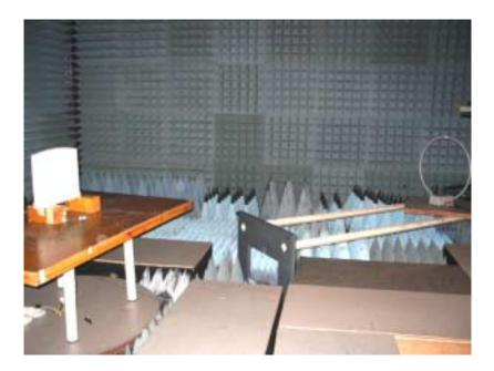
Photograph No.3 Spurious emissions measurement setup in the anechoic chamber in 30 -2900 MHz
