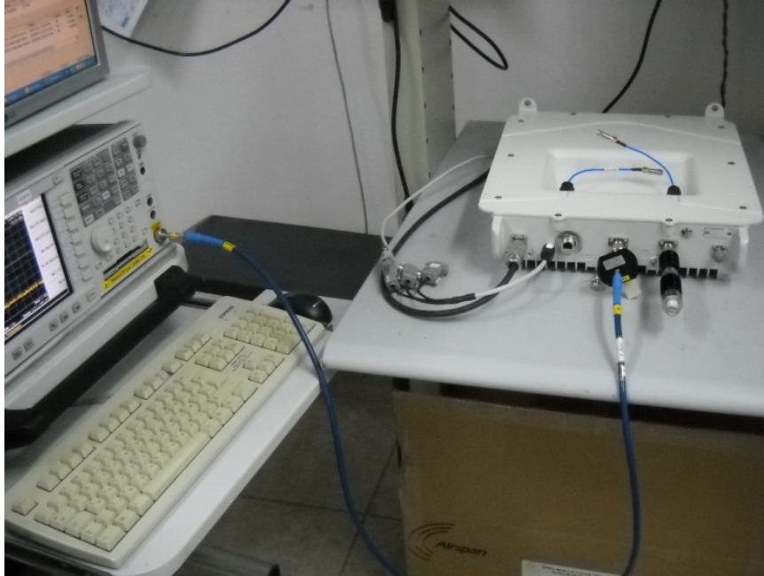
Photograph No.1 Output power, peak spectral density, occupied bandwidth and conducted spurious emissions measurement setup
