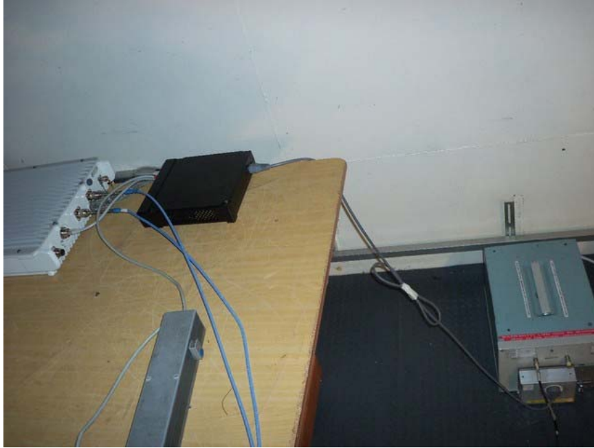
Photograph No.5 Conducted emissions measurement setup on AC power lines
