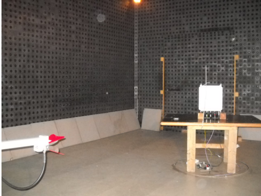
Photograph No.4 Spurious emissions measurement setup in the anechoic chamber above 1 GHz
