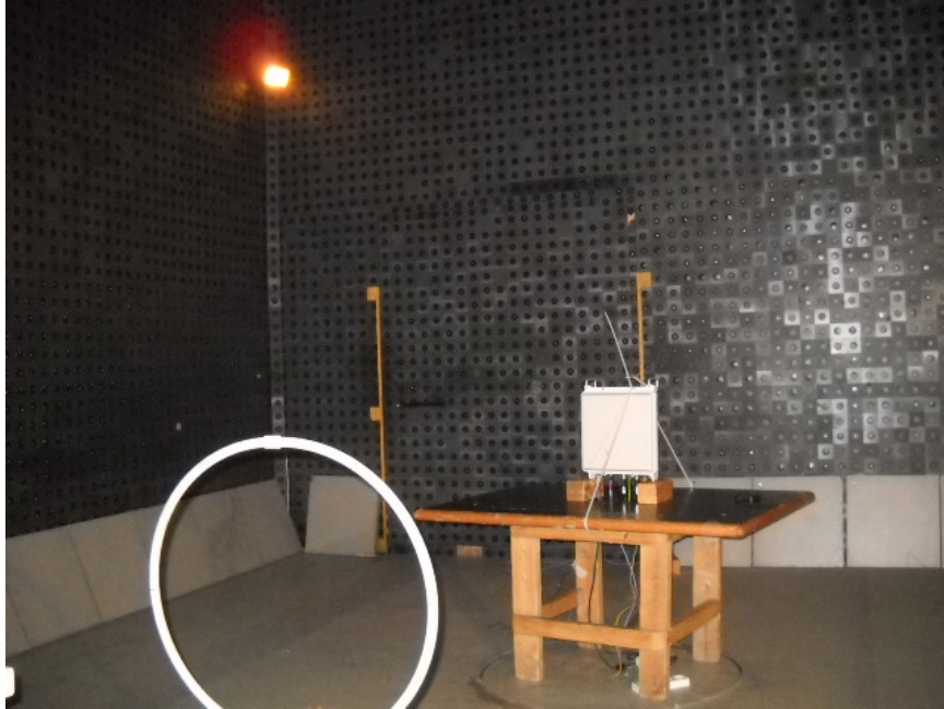
Photograph No.2 Spurious emissions measurement setup in the anechoic chamber below 30 MHz
