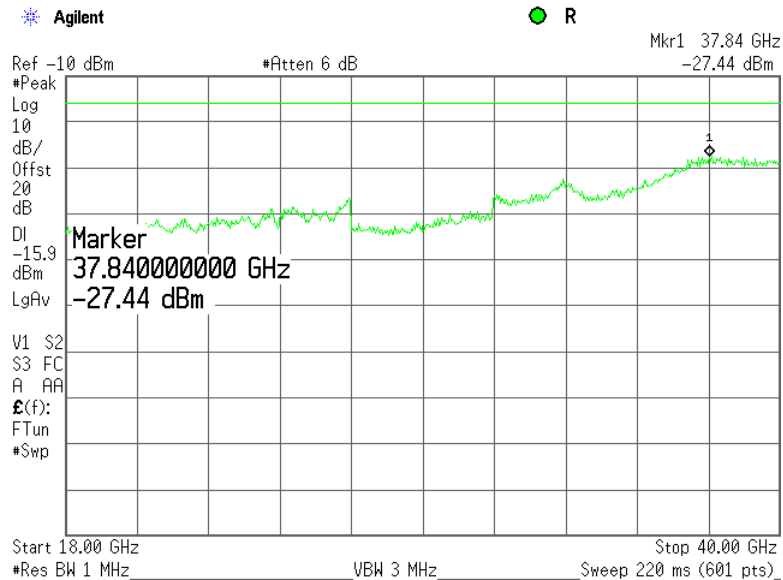
Plot 7.3.18 Spurious emission measurements in 18000 - 40000 MHz range at high carrier frequency
