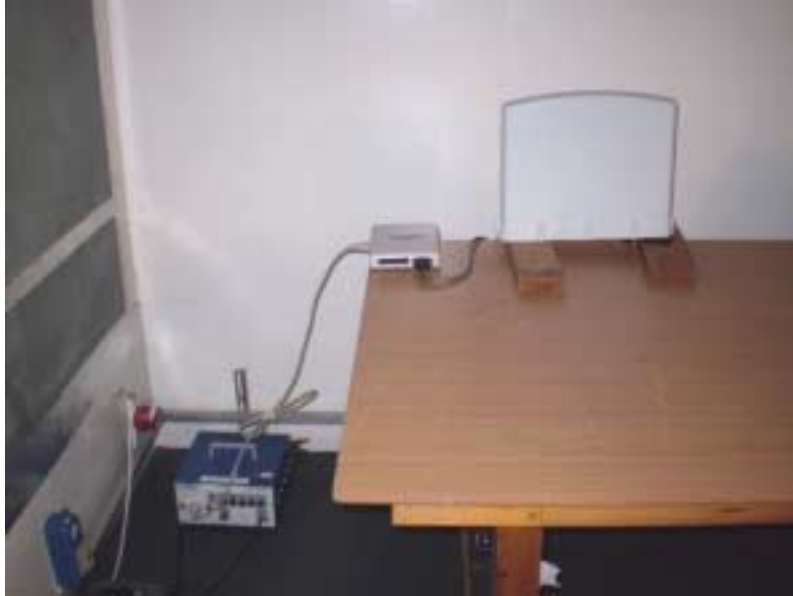
Photograph No.5 Conducted emissions measurement setup on AC line
