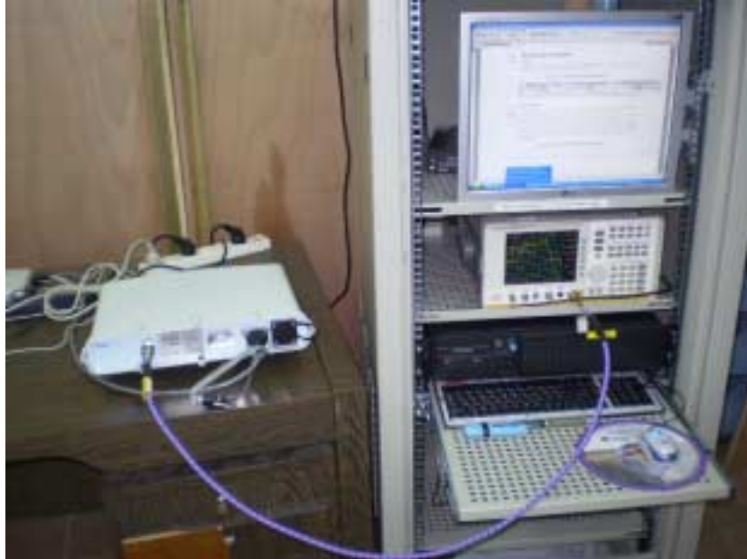
Photograph No.1 Peak output power, power spectral density, occupied bandwidth and conducted spurious emissions measurement setup
