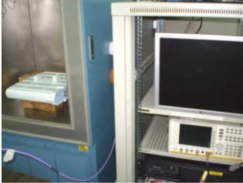
Photograph No.4 Frequency stability test setup
