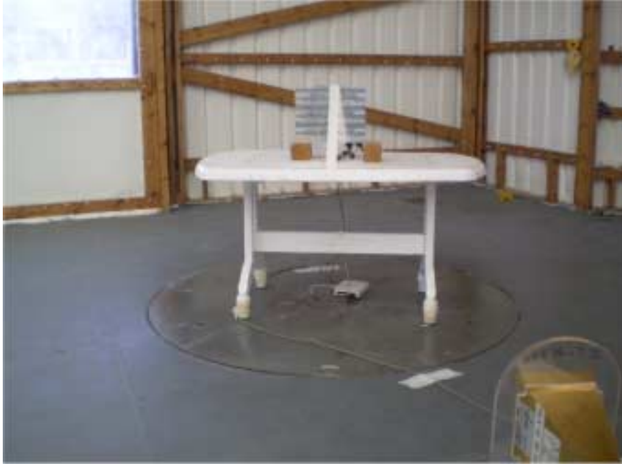
Photograph No.7 Spurious emissions measurement setup at the OATS in 26-40 GHz
