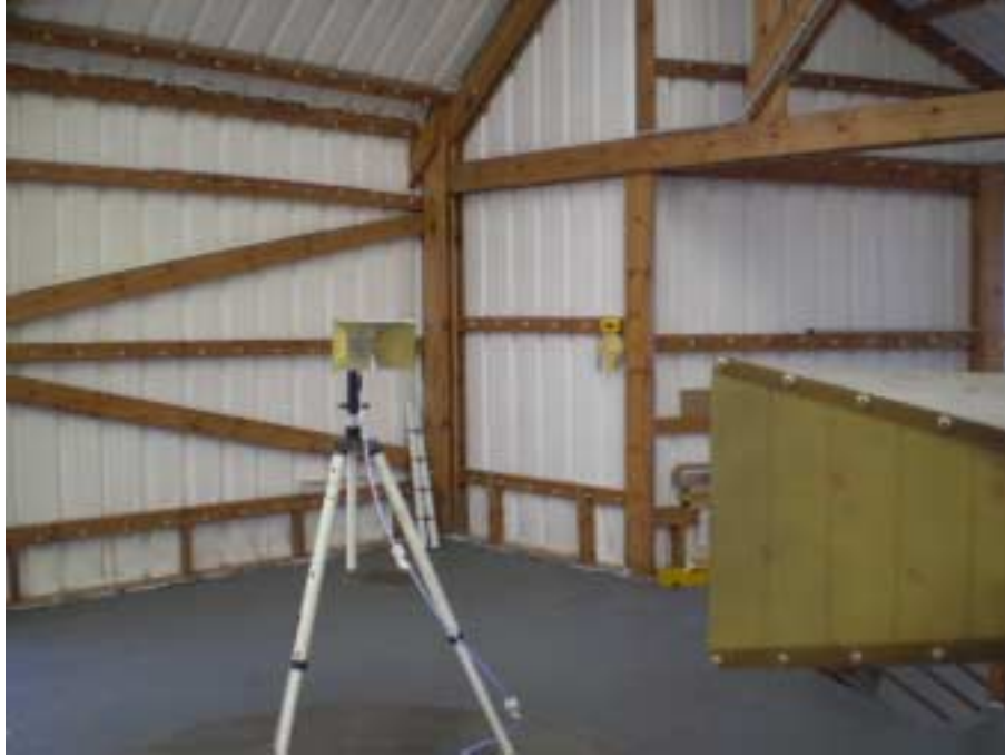
Photograph No.9 Substitution method measurement setup at the OATS above 1000 MHz
