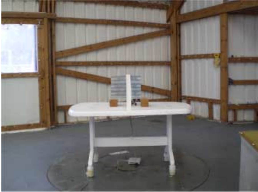
Photograph No.5 Radiated emissions measurement setup at the OATS in 1 - 18 GHz
