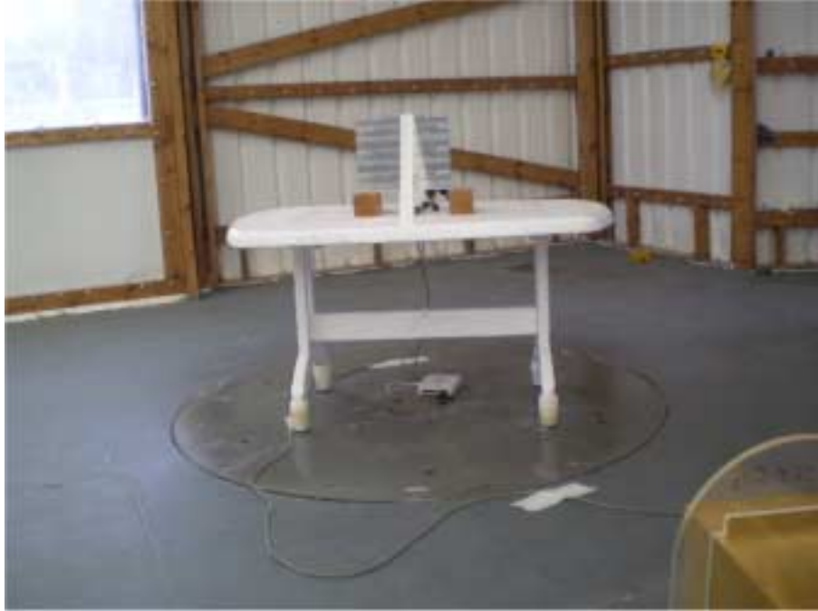
Photograph No.6 Spurious emissions measurement setup at the OATS in 18 - 26 GHz
