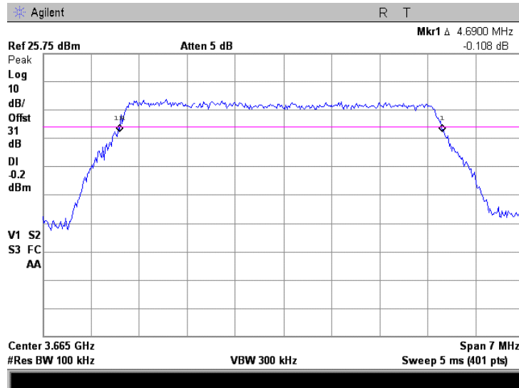
Plot 7.2.6 Occupied bandwidth test result at mid frequency, BPSK, rate 2.095 Mbps
