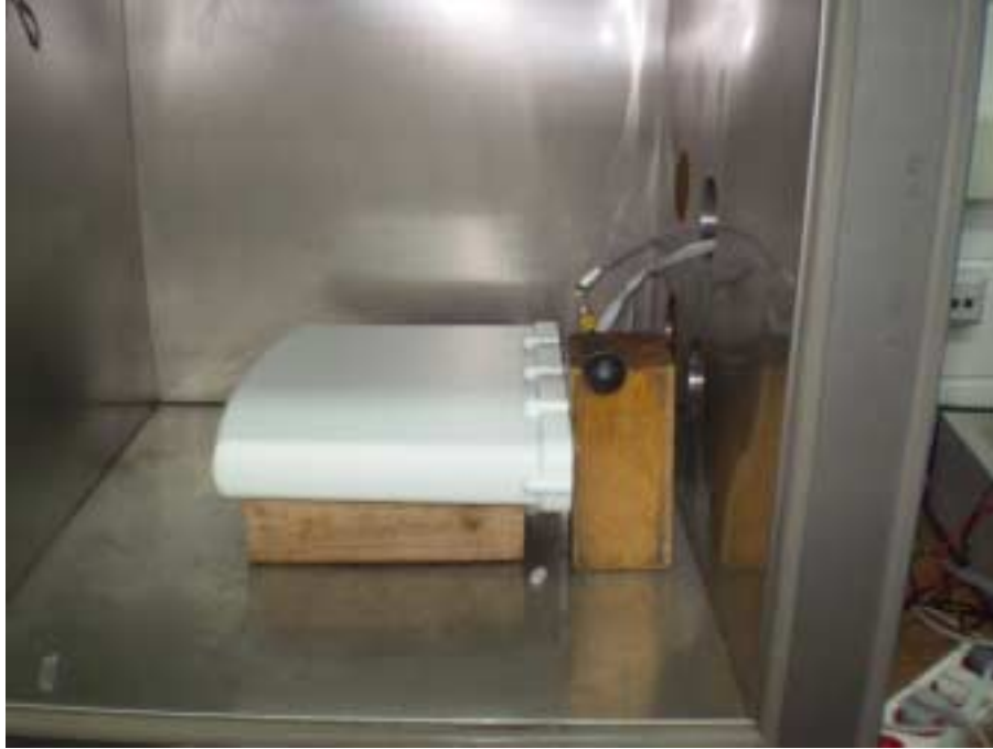
Photograph No.6 Frequency stability measurement setup
