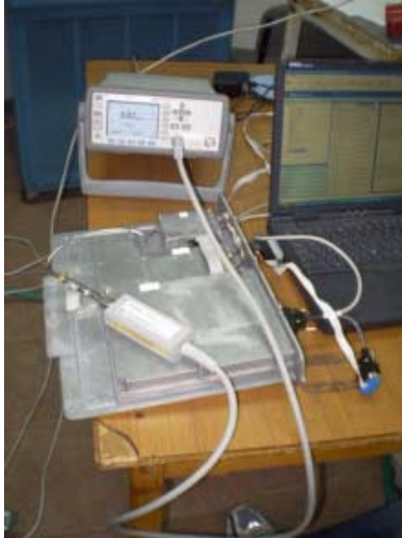
Photograph No.1 Peak output power, power spectral density, conducted spurious emissions measurement setup
