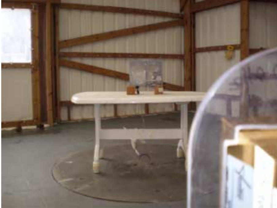
Photograph No.5 Radiated emissions measurement setup on the OATS above 1000 MHz
