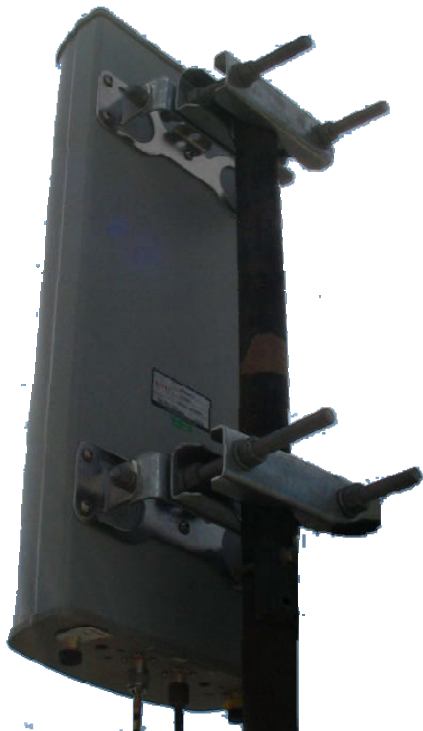
Figure 16 – MacroMAXe Antenna Quad Slant Mast Mount Configuration
