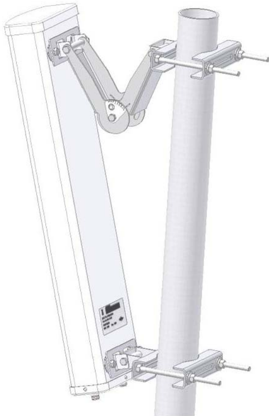
Figure 15 - MacroMAXe Antenna Dual Slant Mast Mount Configuration
