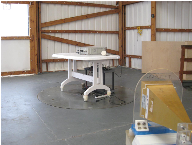
Photograph No.7 Spurious emissions measurement setup at the OATS above 1000 MHz
