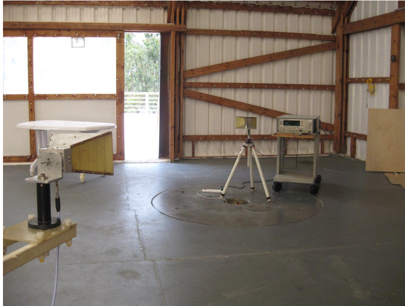
Photograph No.8 Setup for substitution method of spurious ERP measurements
