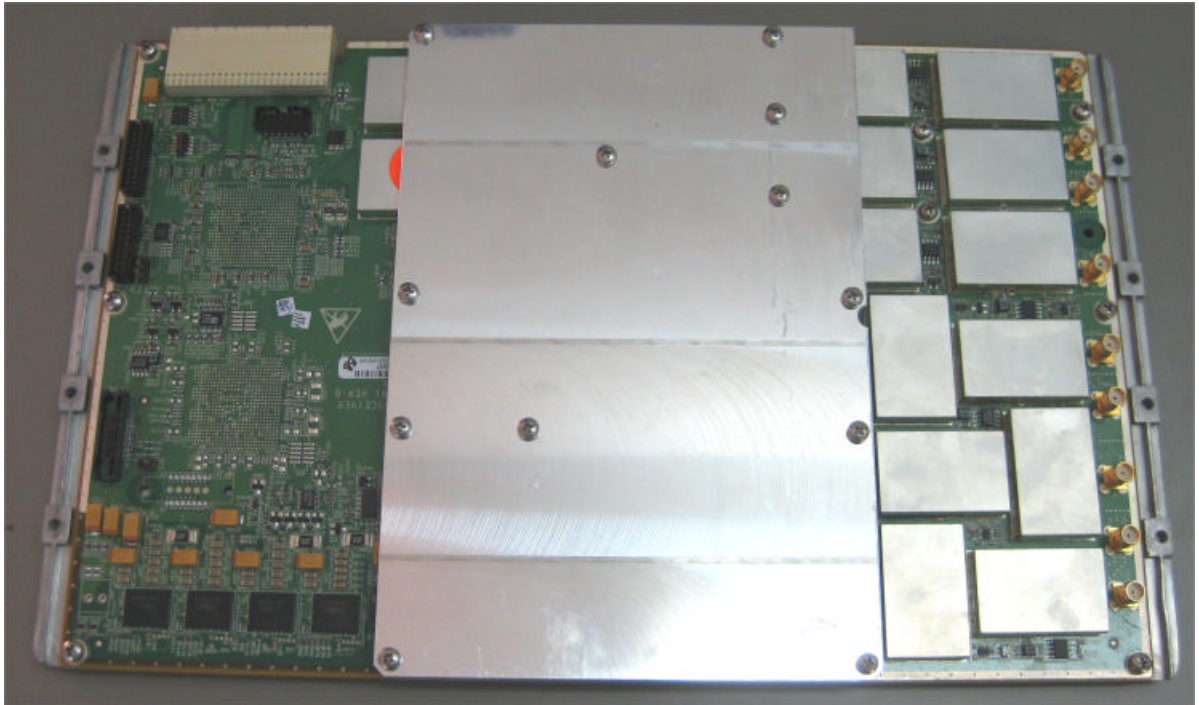
Photograph No.2 “MicroMAXe 3605 3.7 G Ext” RF card front view
