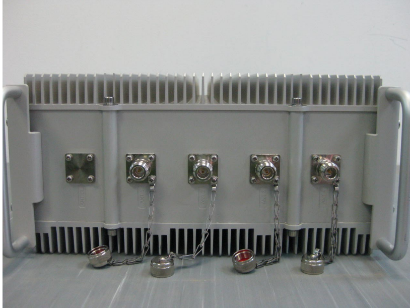
Photograph No.3 “MicroMAXe 3605 3.7 G Ext” antenna connectors view
