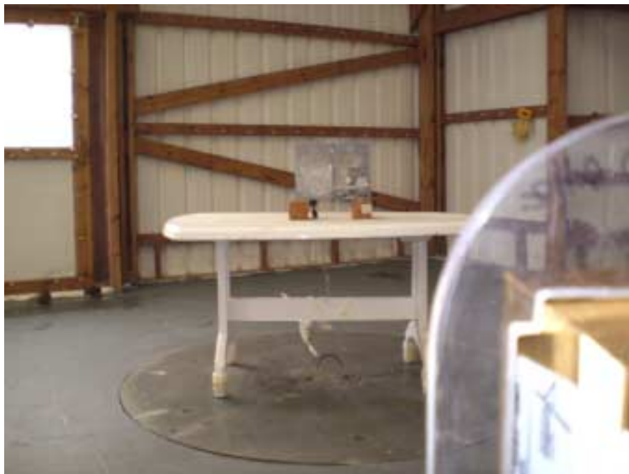
Photograph No.5 Radiated emissions measurement setup an the OATS above 1000 MHz
