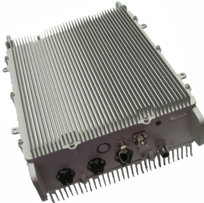
Figure 7 – Air4G-W24 Base Station Unit, Ethernet termination
