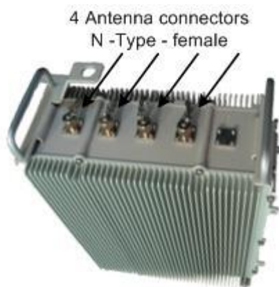
Figure 23 – Air4G-W24 External Antenna Configuration
