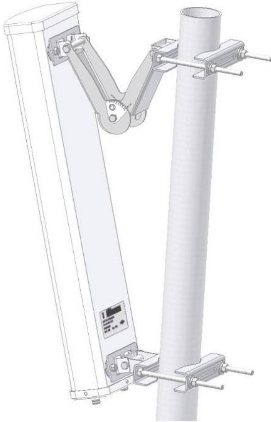
Figure 24 - Air4G-W24 Antenna Dual Slant Mast Mount Configuration
