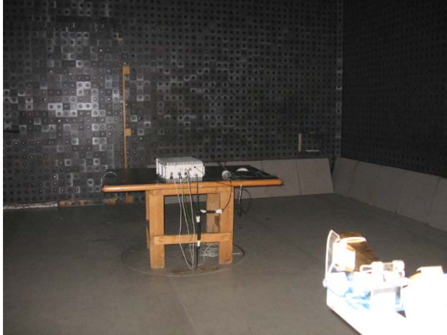
Photograph No.7 Radiated emissions measurement setup in the anechoic chamber in 26.5 –27 GHz range
