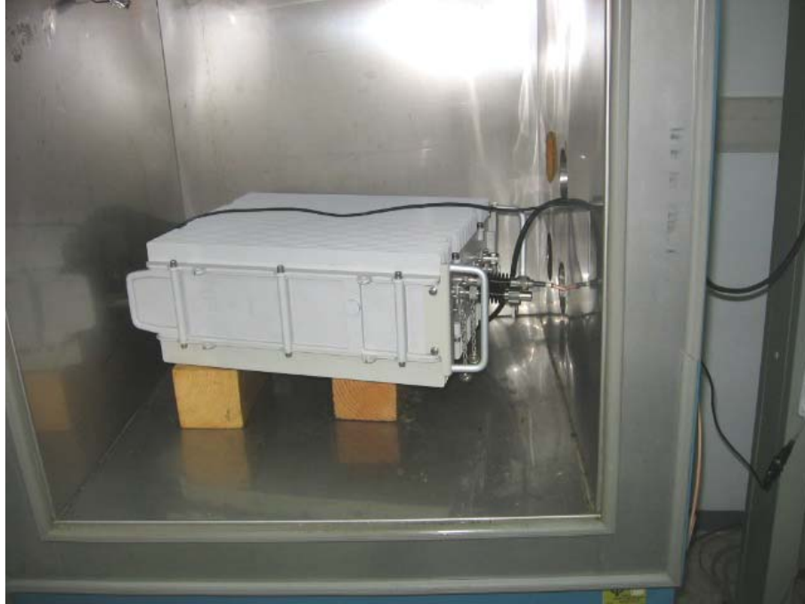
Photograph No.9 Frequency stability measurement setup
