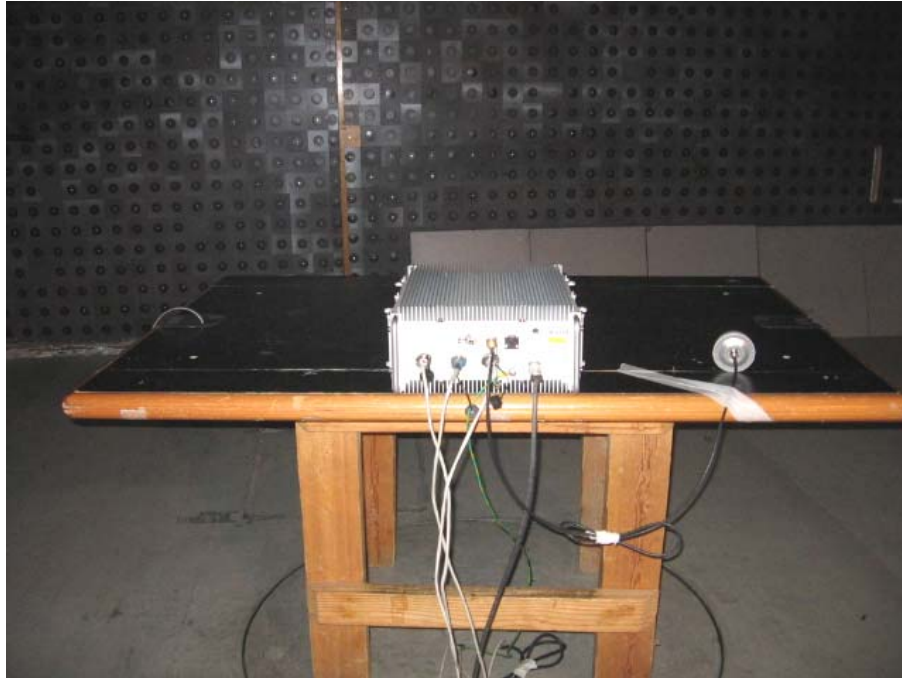
Photograph No.8 Radiated emissions measurement setup in the anechoic chamber, EUT close view
