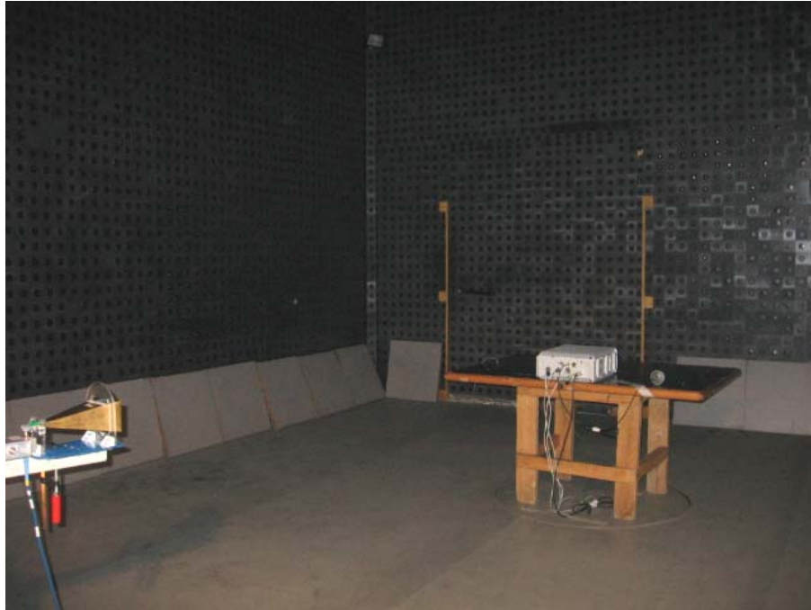
Photograph No.6 Radiated emissions measurement setup in the anechoic chamber in 18-26.5 GHz range
