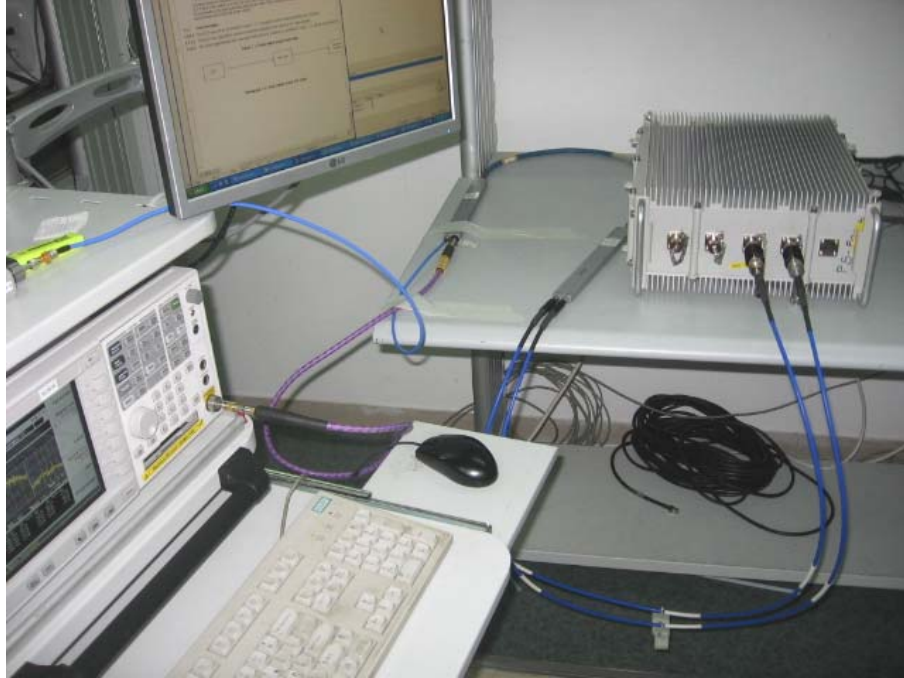
Photograph No.2 Emission mask and conducted spurious emissions measurement setup
