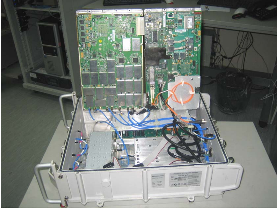
Photograph No.1 “MacroMAXe 2510H” internal view
