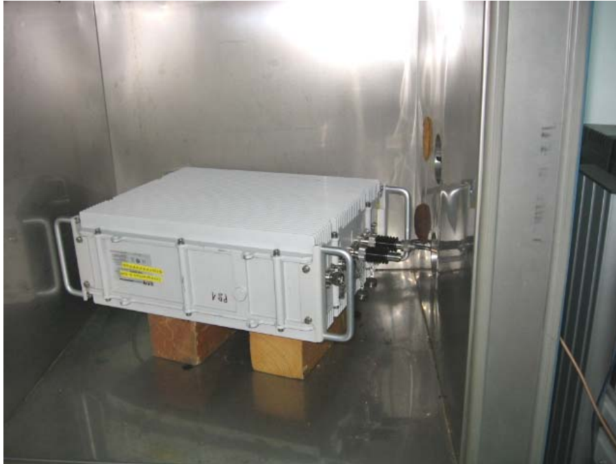
Photograph No.8 Frequency stability measurement setup
