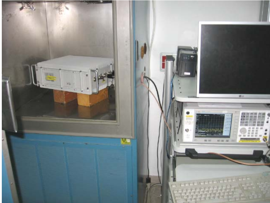
Photograph No.9 Frequency stability measurement setup
