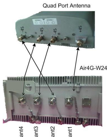
Figure 31 - Quad port antenna connection – 1
