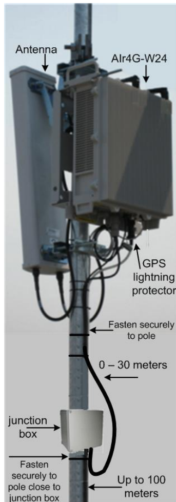
Figure 38 - Air4G-W24 assembly with optional junction box
