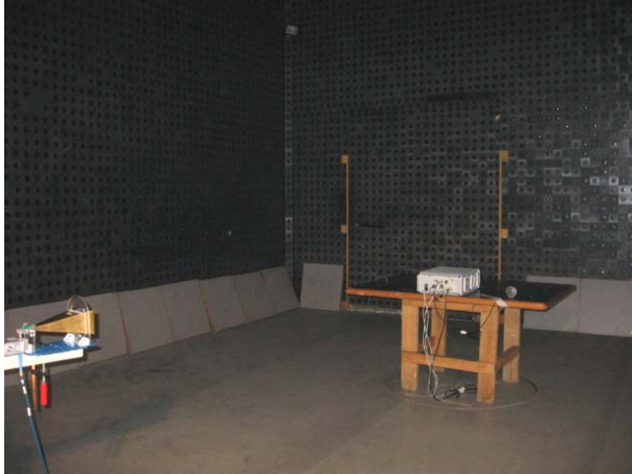
Photograph No.6 Radiated emissions measurement setup in the anechoic chamber in 18-26 GHz range
