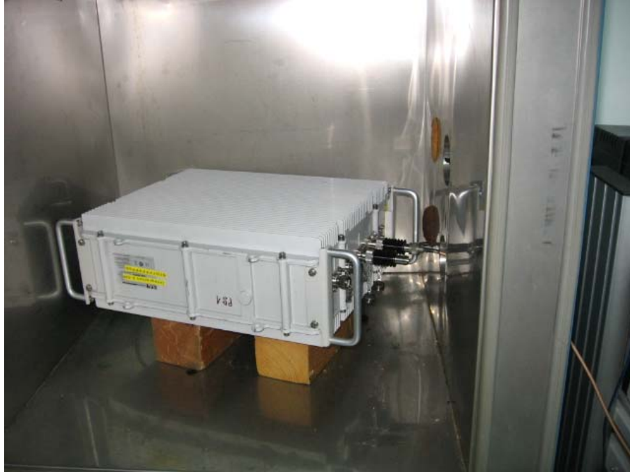
Photograph No.8 Frequency stability measurement setup
