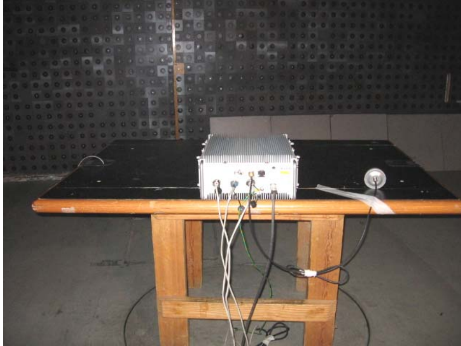
Photograph No.7 Radiated emissions measurement setup in the anechoic chamber, EUT close view
