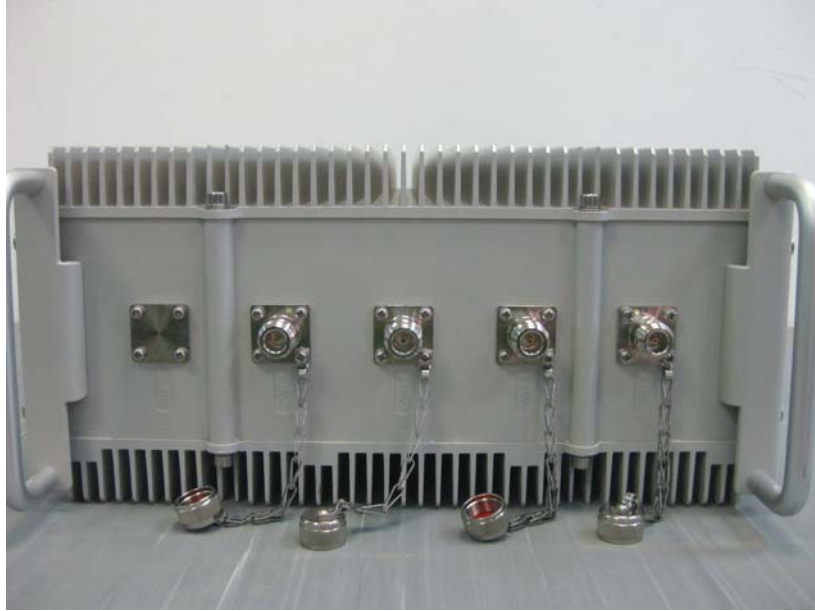
Photograph No.3 “MacroMAXe 2510L” antenna connectors view
