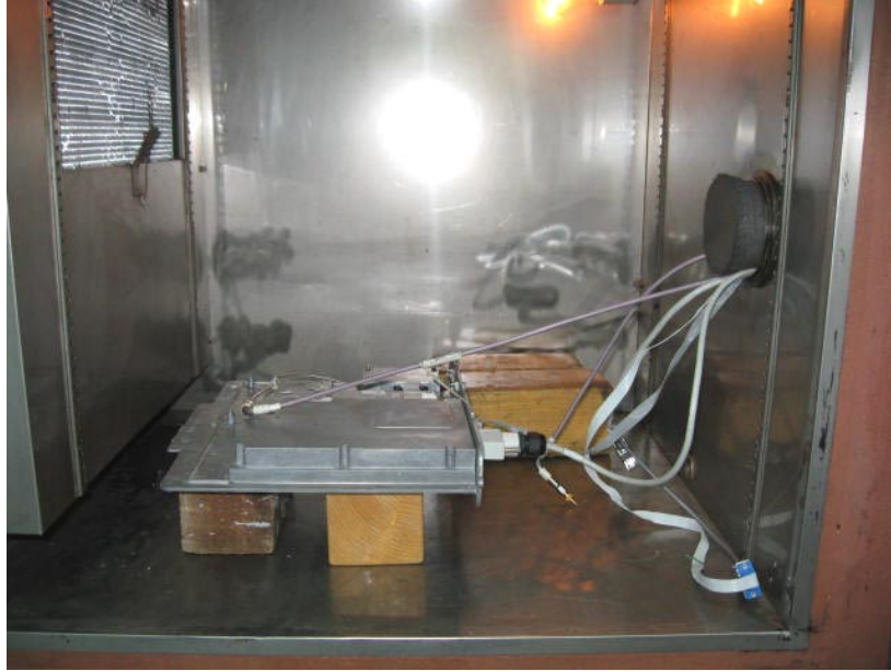
Photograph No.7 Frequency stability measurement setup
