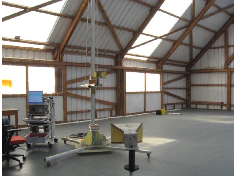
Photograph No.6 Setup of substitution ERP measurements of spurious at the OATS
