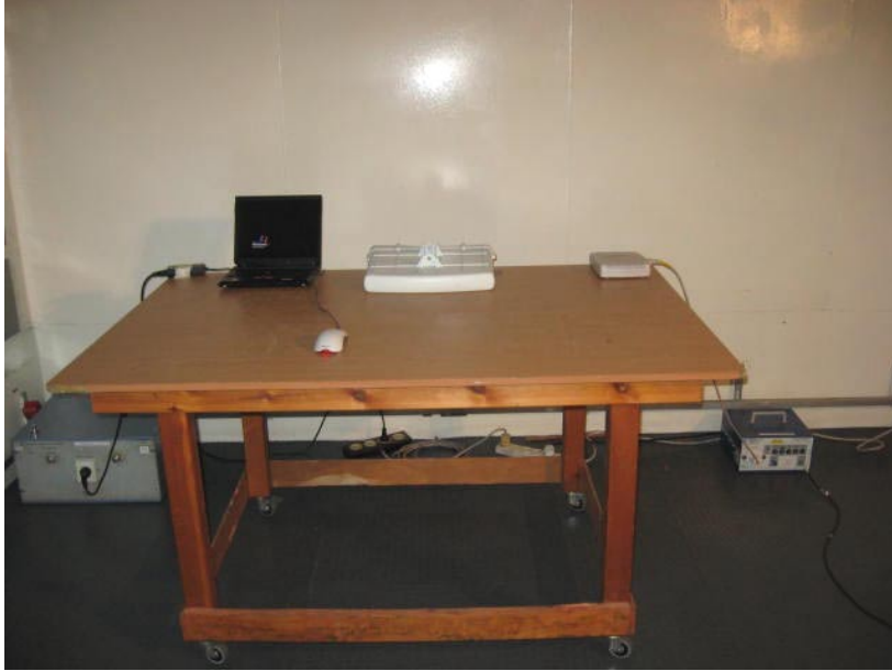
Photograph No.8 Conducted emissions measurement on AC line setup
