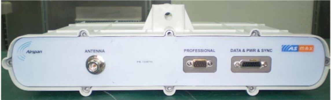
Photograph No.4 MicroMAX 2.5G TDD bottom view
