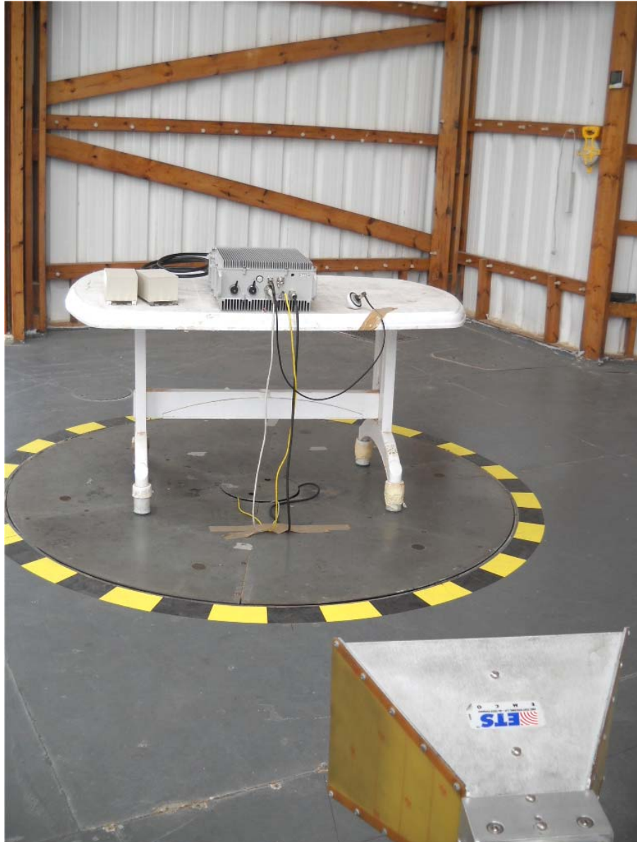
Photograph No.7 Spurious emissions measurement setup at the OATS
