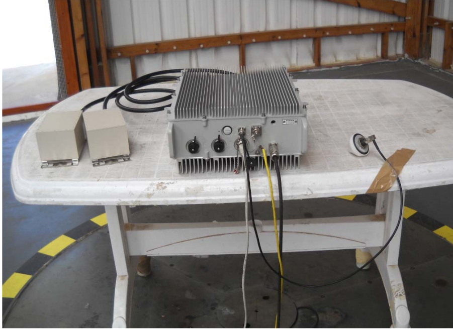
Photograph No.8 Spurious emissions measurement setup at the OATS, EUT close view
