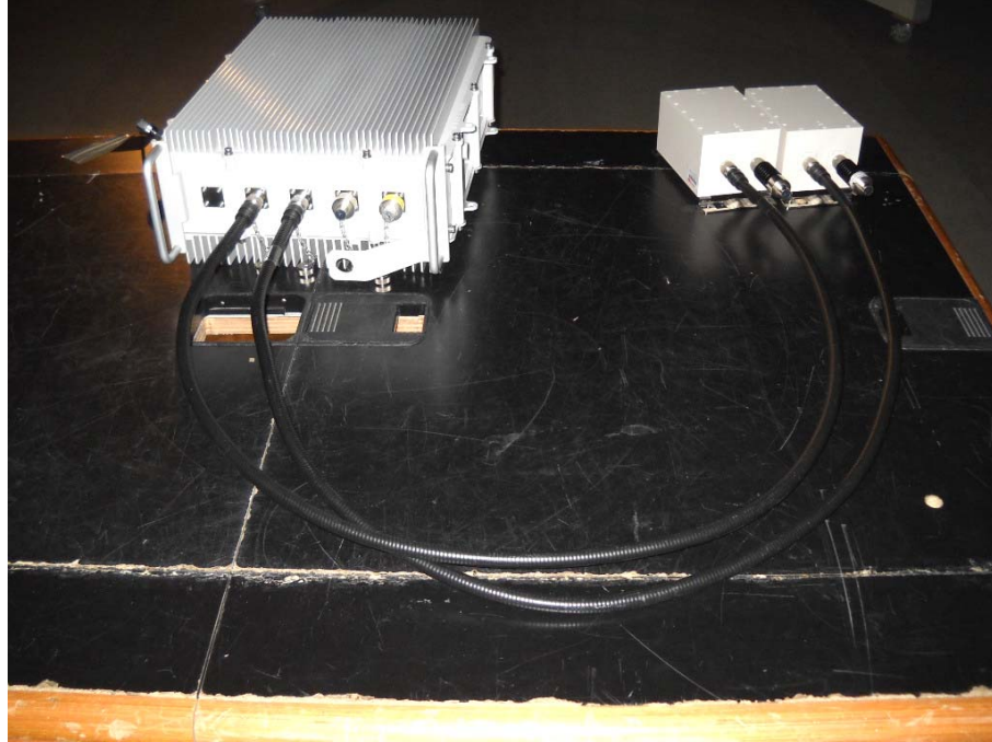
Photograph No.5 Radiated emissions measurement setup in the anechoic chamber, EUT close view
