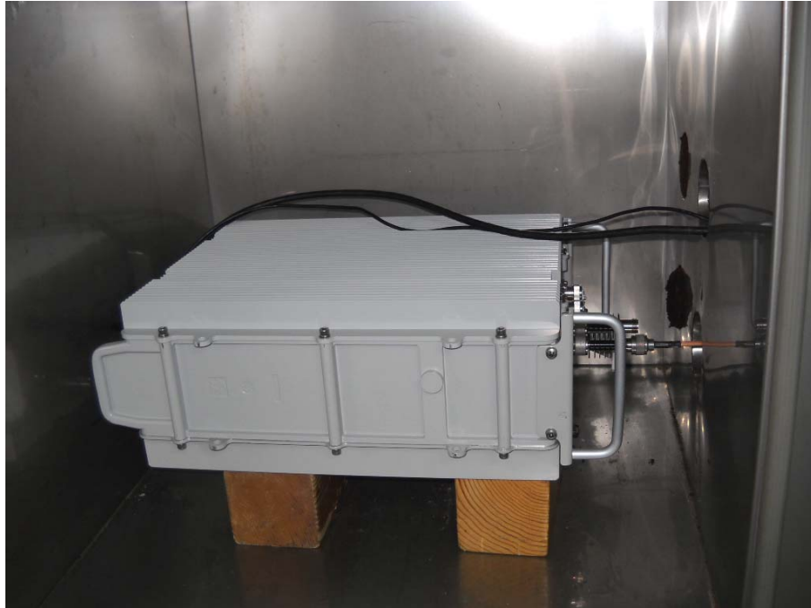
Photograph No.9 Frequency stability measurement setup
