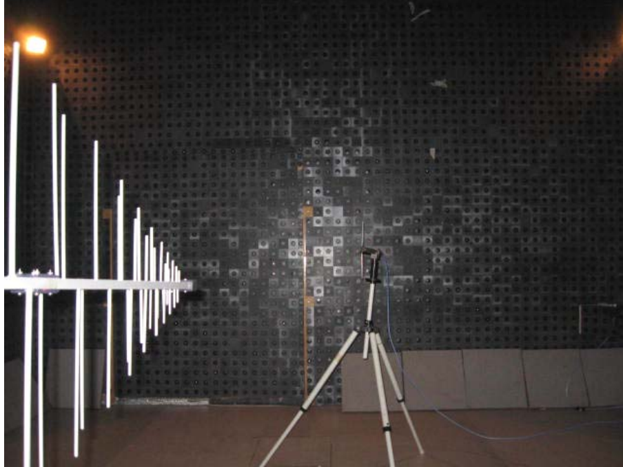
Photograph No.6 Setup for substitution ERP measurements of spurious
