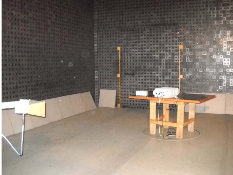
Photograph No.4 Spurious emissions measurement setup in the anechoic chamber in 1-18 GHz range
