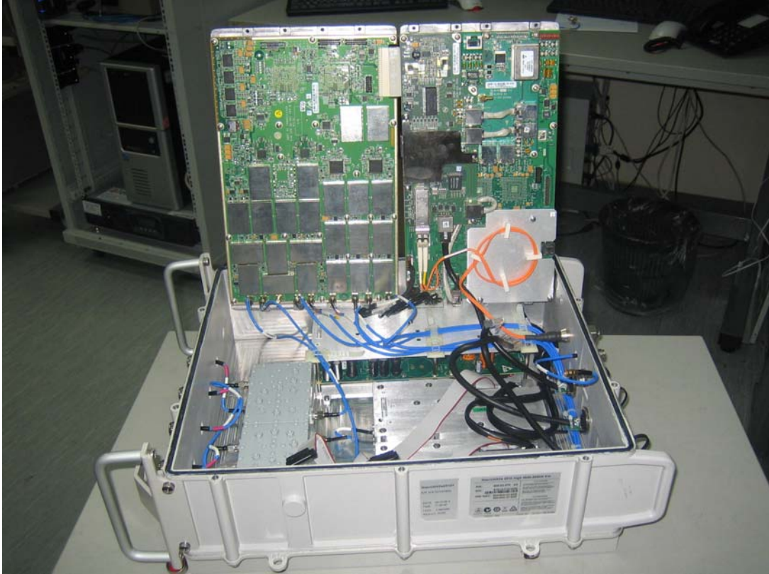
Photograph No.1 “Air4G-MacroMAXe 2310L” internal view
