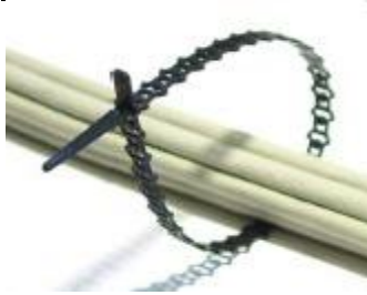
Figure 47 - Secure fiber-optic cable, place tie
