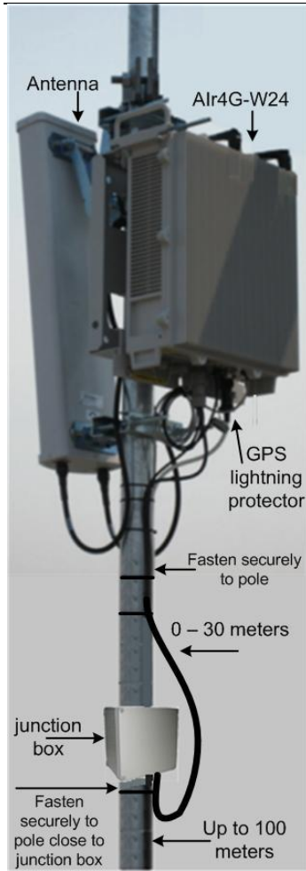
Figure 39 - Air4G-W24 assembly with optional junction box
