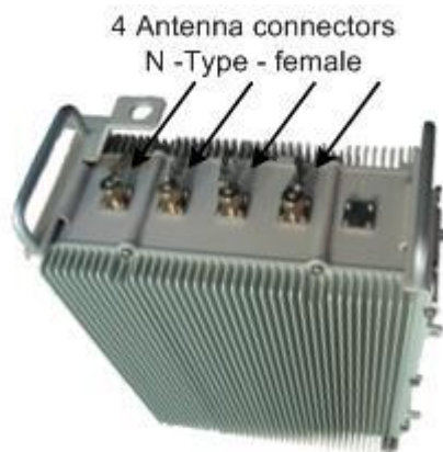
Figure 23 – Air4G-W24 External Antenna Configuration
