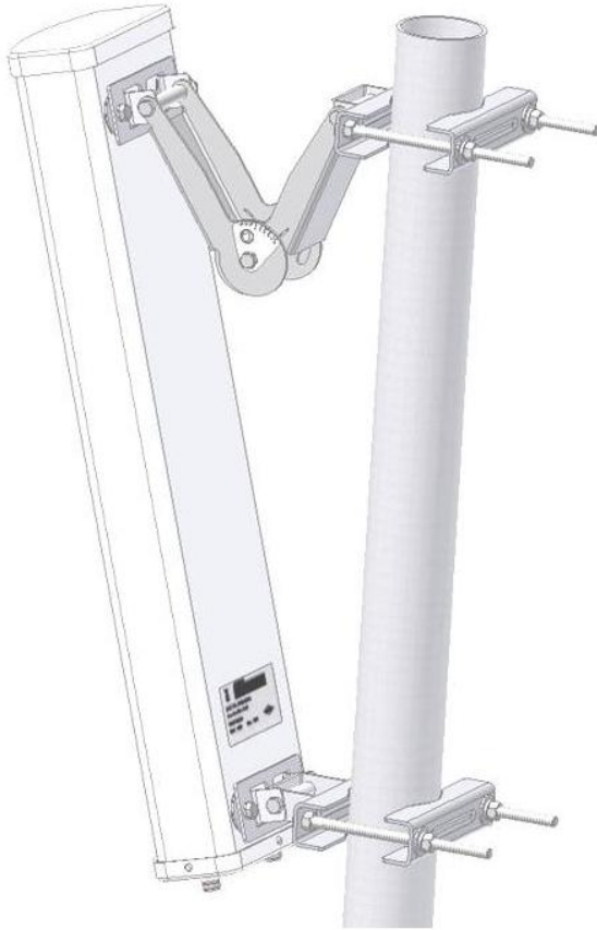
Figure 24 - Air4G-W24 Antenna Dual Slant Mast Mount Configuration
